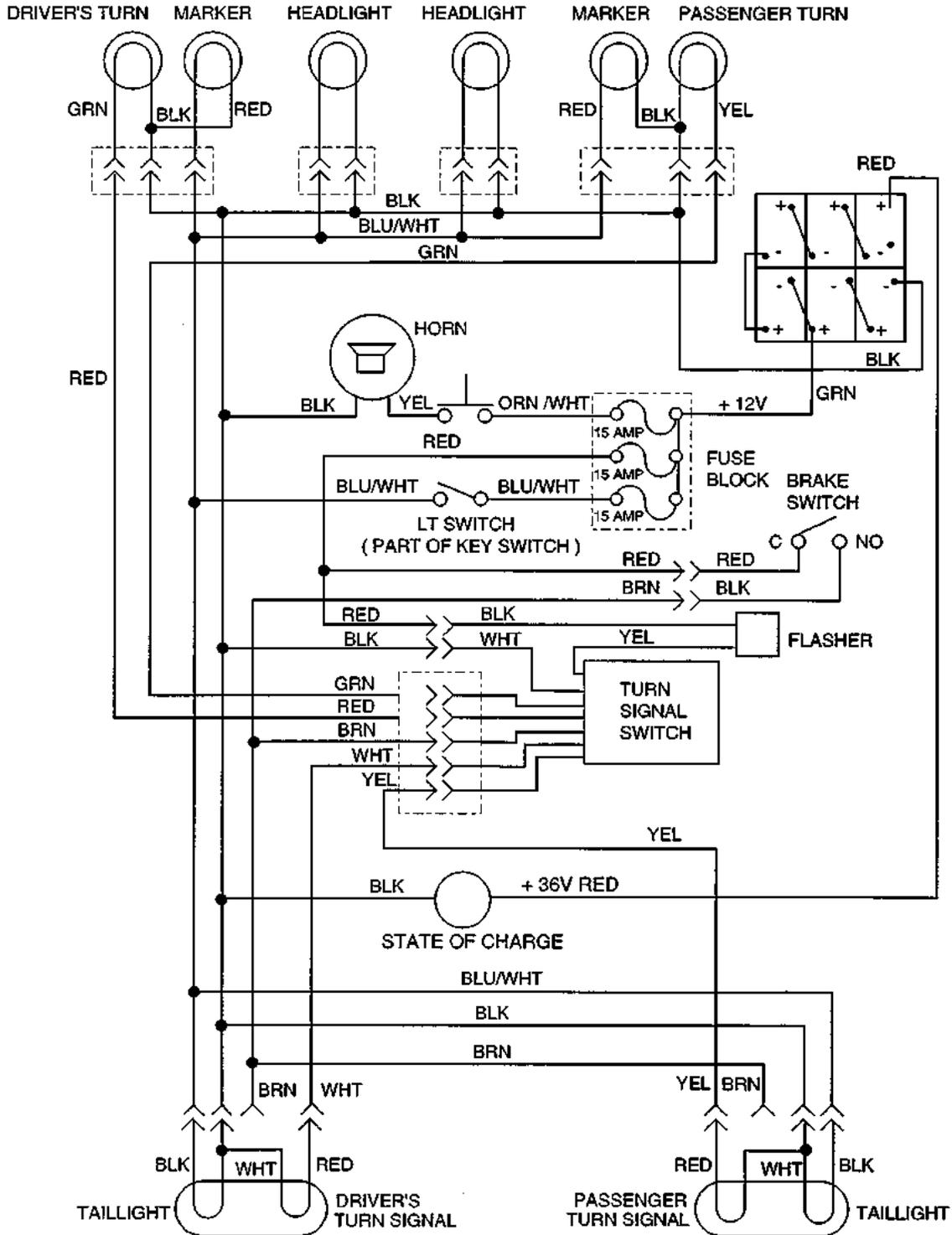
FOR VEHICLES WITHOUT TURN SIGNALS REMOVE WHT WIRE FROM LEFT TURN SIGNAL
